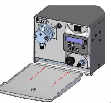
The drip tray is to be installed in the slot near the bottom of the pump.
