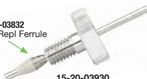
15-20-03930 EXP Nut & Ferrule Hand-tight to 8,700 PSI Wrench-tight to 20,000 PSI
