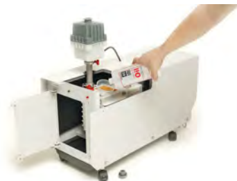
Adding foreline pump (rotary pump) oil, 4 L
