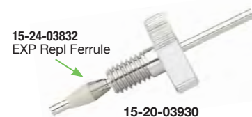
15-20-03930 EXP Nut & Ferrule Hand-tight to 8,700 PSI Wrench-tight to 20,000 PSI
